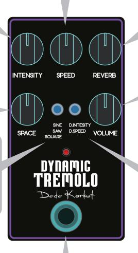
Reverb controls the reverb wet mix from zero at minimum to full reverb at maximum.
